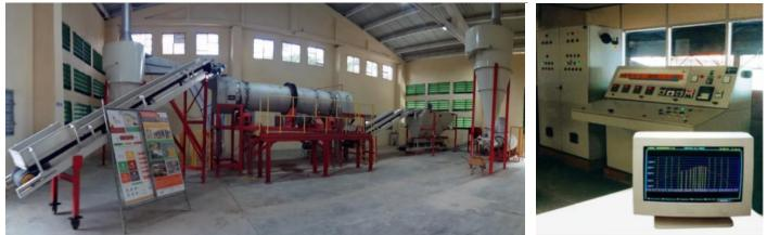
Potential set up for the demonstration plant – 2,000k/hr calcinated clay line. Source: IPIAC
