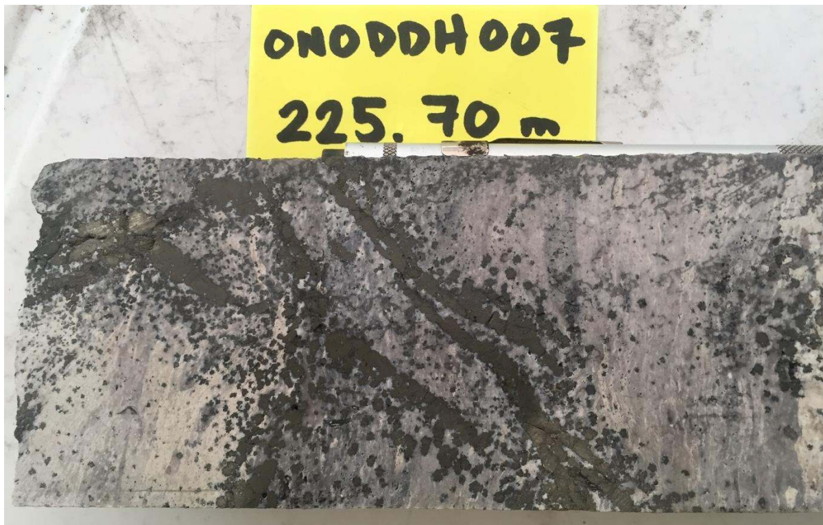
Plate 4 – Altered and mineralized volcanic host rock with up to 7% metallic sulphide in drill hole ONODDH007, HQ core from 225.7 m depth - Ono Island Project, Fiji
