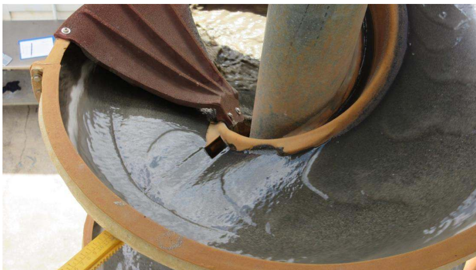
Plate 2 – Darker heavy minerals (including magnetite) are concentrated toward the centre of the spirals, where they are separated for recovery.
