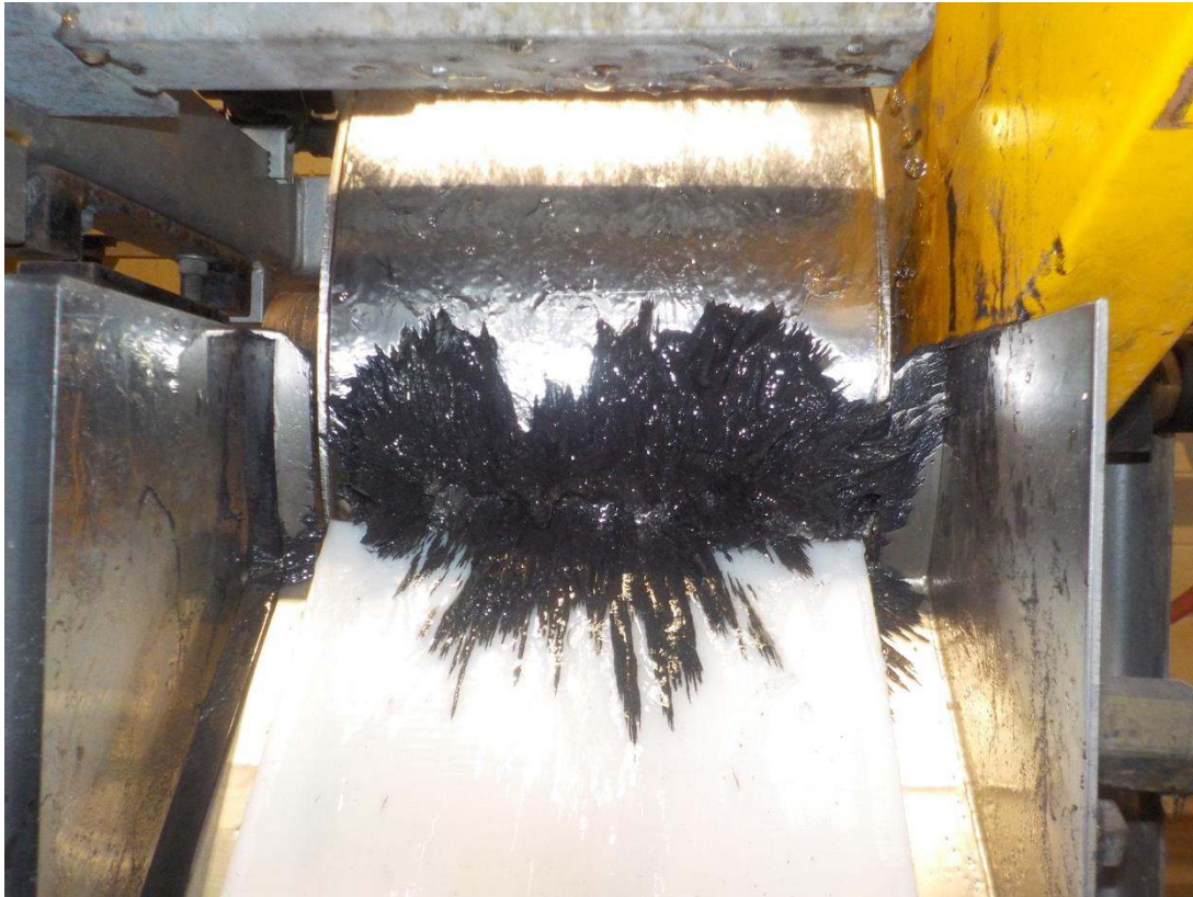
Plate 3 – Titano-magnetite from Sigatoka bulk samples being recovered in a Low Intensity Magnetic Separator test (LIMS).
