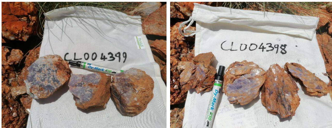
Figure 14: Samples of coarse spodumene (LHS) and coarse lepidolite (RHS) from samples sent for assay.
