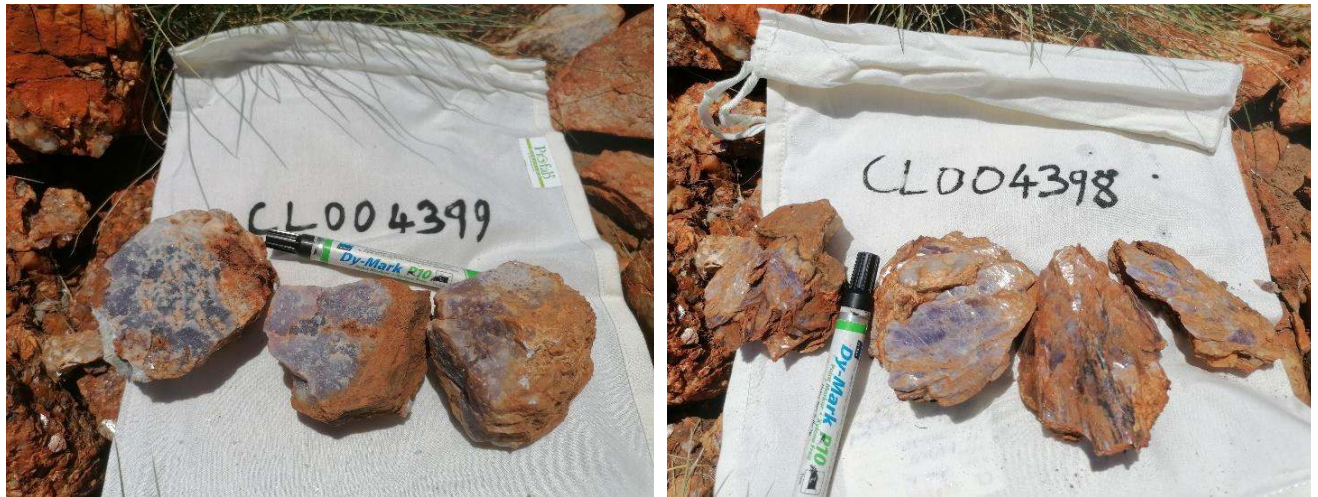
Figure 10: Samples of coarse spodumene (LHS) and coarse lepidolite (RHS) from samples sent for assay.
