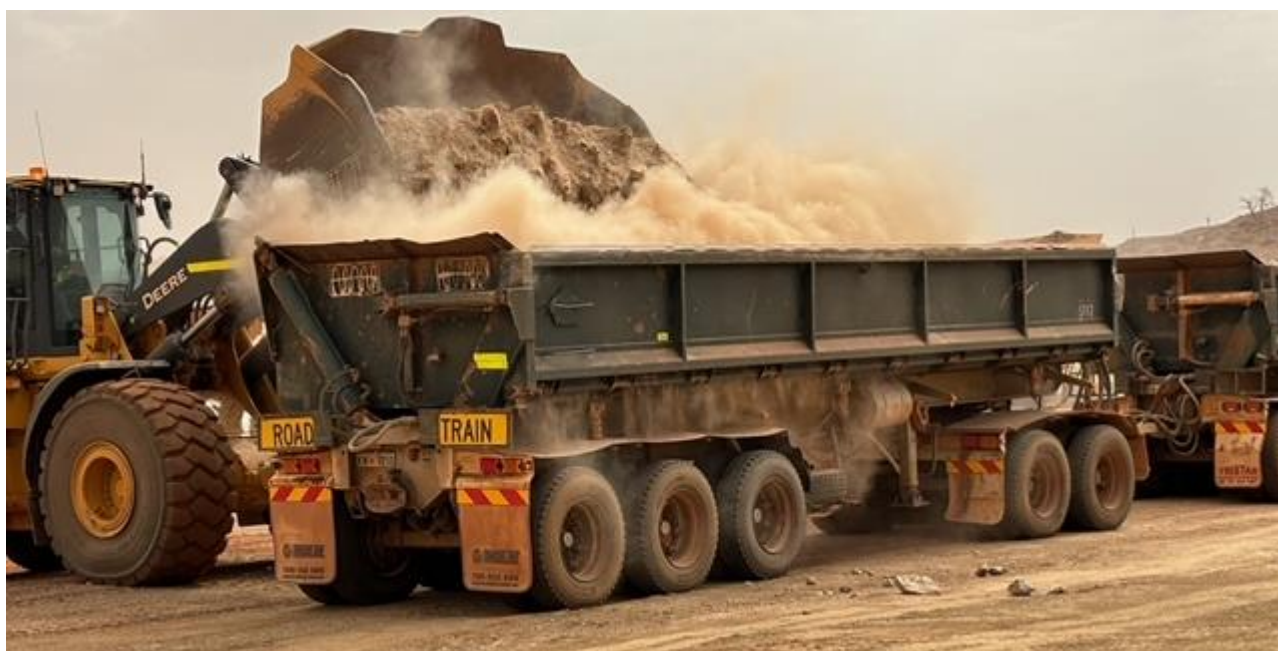
Figure 2: Blue Bar Ore being loaded for trucking to Calidus Resources Processing Plant at Warrawoona.
